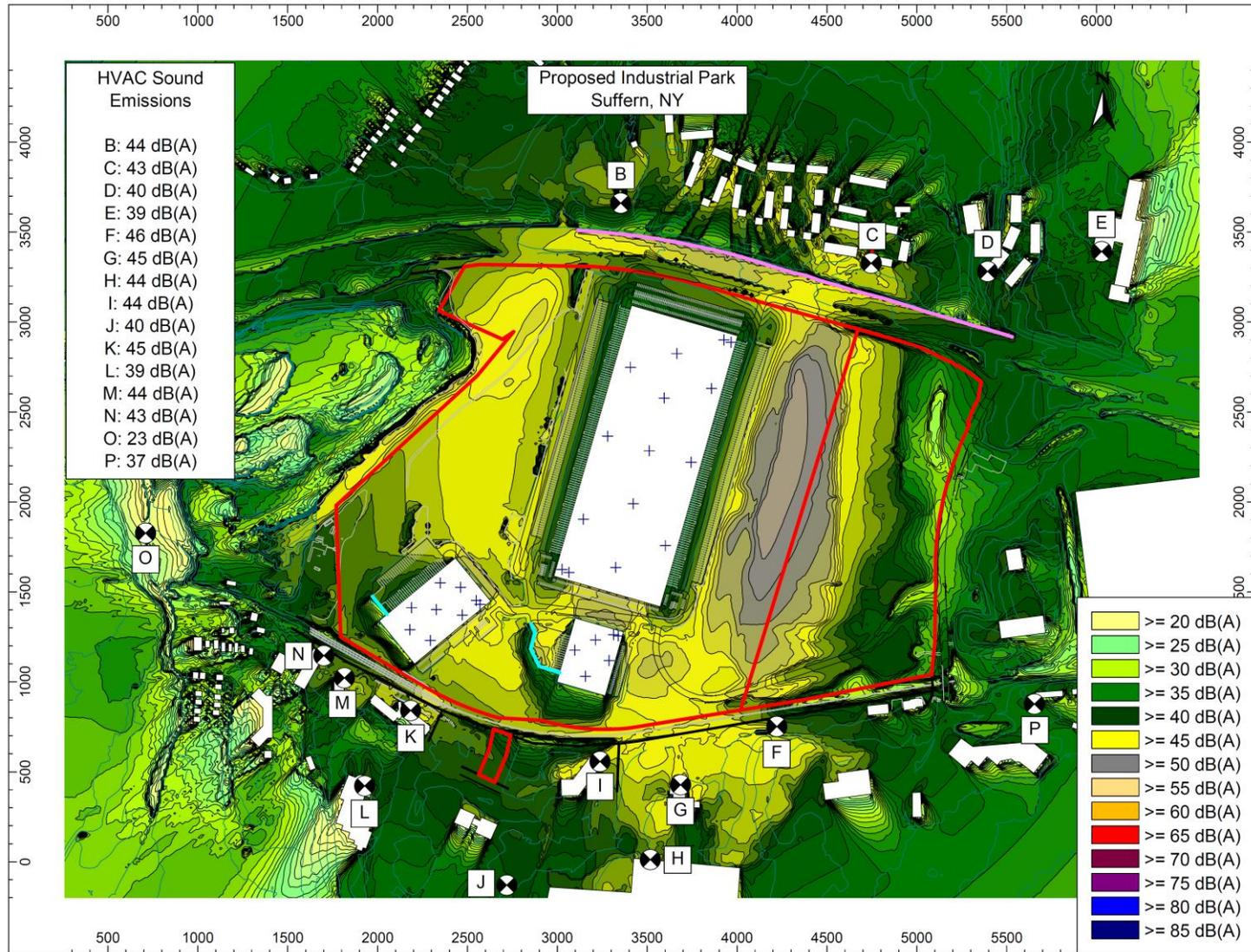
**Figure 2 — A-weighted sound emission contours, 5 feet above grade, from rooftop HVAC equipment. Each HVAC unit shown with a blue + sign. Buildings shown in white, site property line outlined in red, 15-foot-tall sound barrier shown in light blue, and highway sound barrier shown in pink. All Locations typify upper story receptors of interest. See Table II for receptor Location description and modelled height.**
