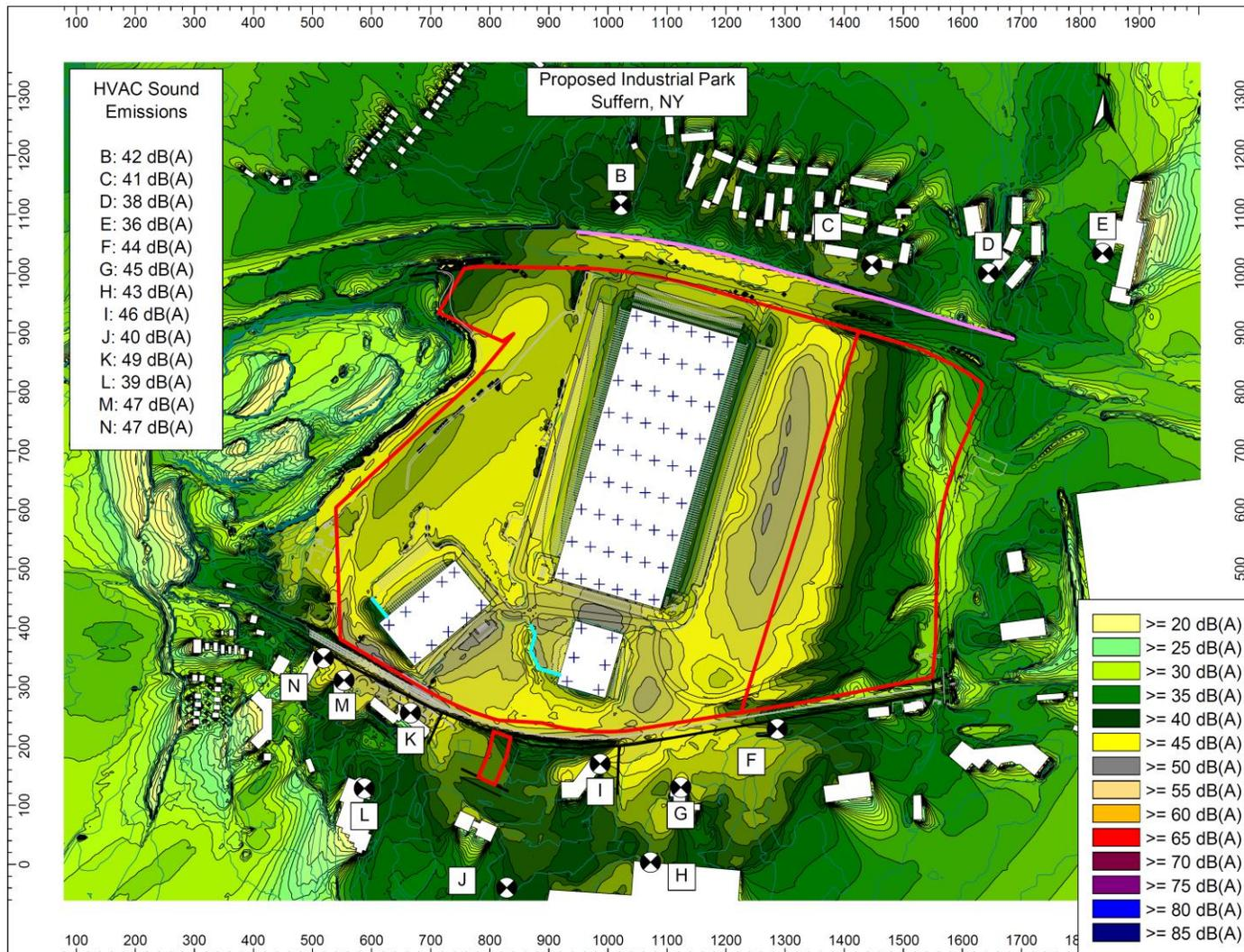
Figure 2 — A-weighted sound emission contours, 5 feet above grade, from rooftop HVAC equipment. Each unit shown with a blue + sign. Buildings shown in white, site property line outlined in red. **All Locations typify upper story receptors of interest.** See Table 1 for Location description and modelled height.
